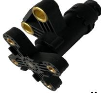
Used in the ECAS system. Used to determine the value of movement. Technical specifications Bayonet: DIN 72585-A1-2.1-Sn / K2. AC voltage: 8-16 V. Measuring principle: inductive. Current consumption, max: 90mA. Operating temperature, ° C: from minus 40 to plus 80 Working environment: air. Analog: Wabco441 050 121 0
