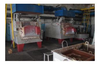
Carbonitriding in the electric furnace. The maximum temperature 950°C. Power 63 kW. Capacity of the furnace 150 kg/hour. The size of furnace working space Ø 600x600 mm.
