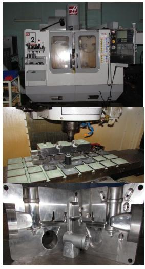
Production of molds: for molding under pressure of aluminium alloys for injection molding of plastics for the manufacture of rubber goods.
